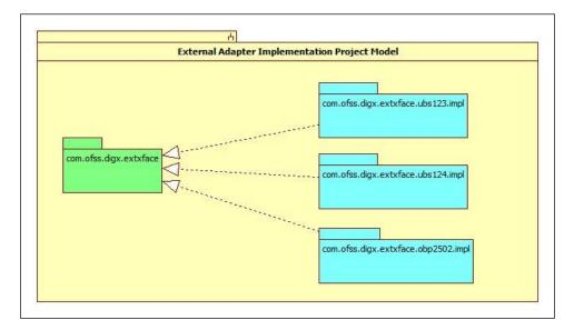
In above model, project **com.ofss.digx.extxface** contains all the adapter specifications (Java Interface) for external facing adapters. The concrete implementation classes of the adapter interfaces will reside in the host specific adapter implementation project.
